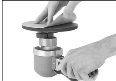
**Figure 9.** Attaching sanding disc.
