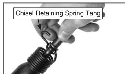
**Figure 3.** Chisel installation.
