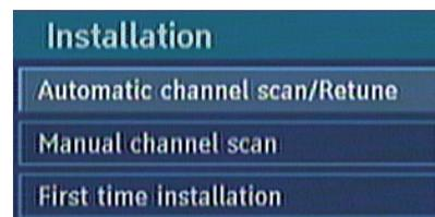
Automatic channel scan is activated by selecting OK when the line is highlighted. A pop-up menu appears on the screen, select "YES" the automatic scan begins. All the multiplexes are searched and a channel table is created automatically. All channels found are stored in a sorted form with respect to their channel numbers. Selecting "NO" will cancel the operation.
