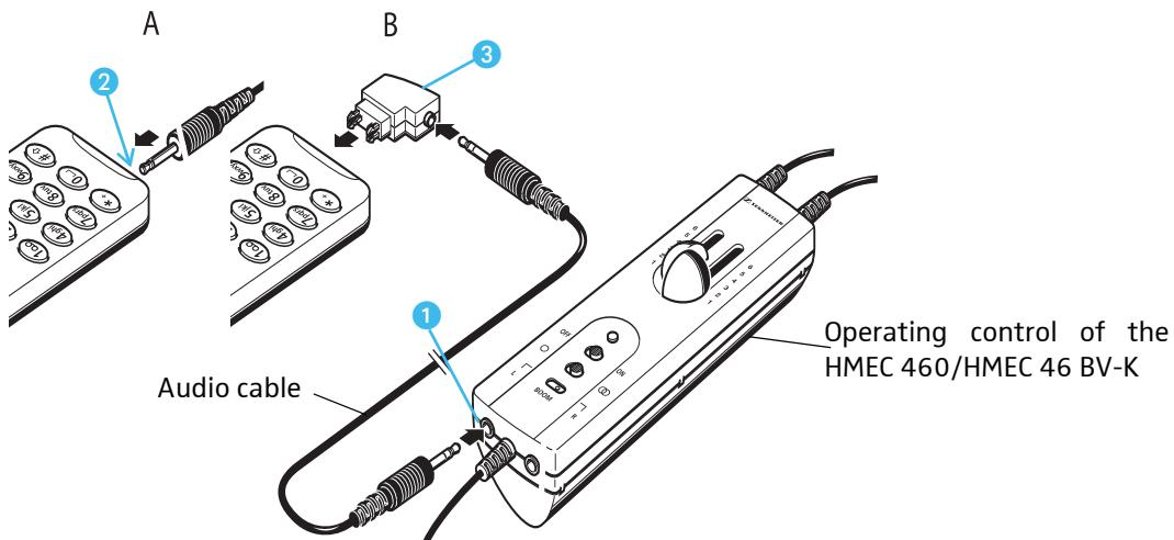
Via an audio cable, you can connect a mobile telephone to the following aviation headsets from Sennheiser:
