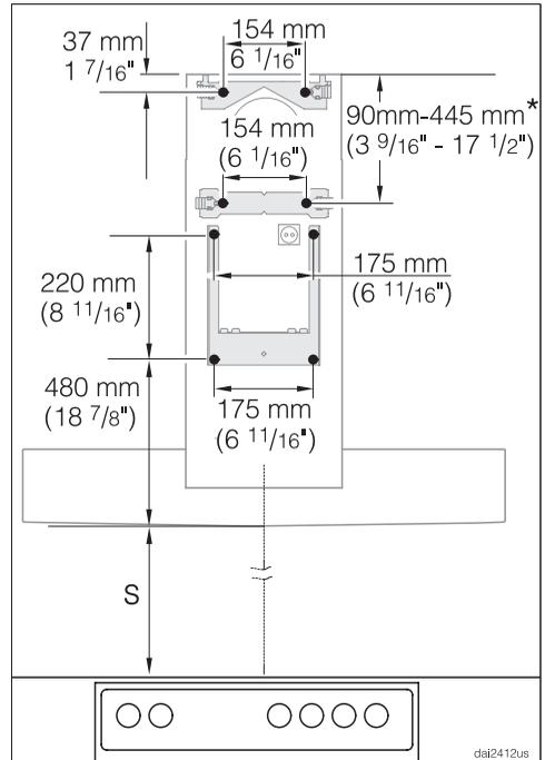
\*The middle retaining plate can vary in position, depending on the ventilation gap and the position of the outlet. It should be mounted as low as possible.
