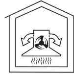
Air is drawn through the grease filter and **active charcoal filter**. The filtered air is then recirculated back into the kitchen through a vent at the top of the hood's chimney.
