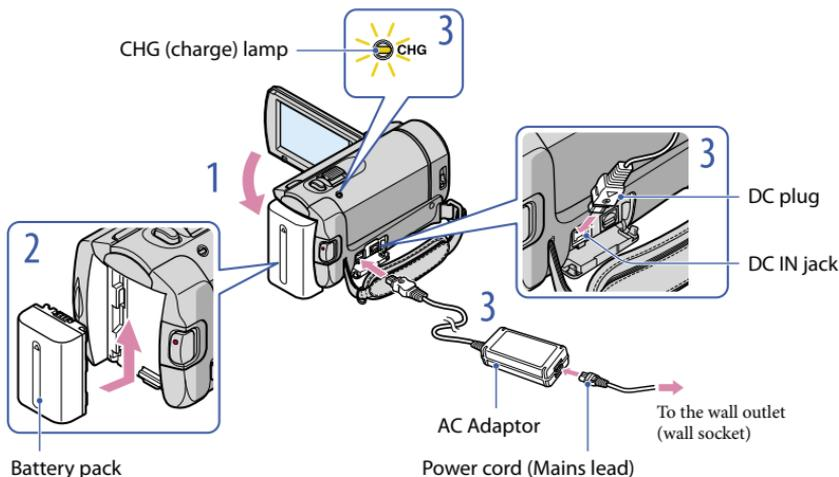
You can charge the “InfoLITHIUM” battery pack (H series) after attaching it to your camcorder.
