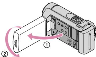
Open the LCD panel 90 degrees to the camcorder ①, then rotate it 180 degrees to the lens side ②.
