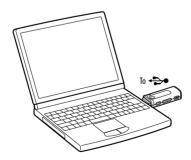
When the remaining battery indication of the display shows: **[Full**], charging is complete. When you use the player for the first time, or if you have not used the player for a long time, recharge it fully until **[Full**] appears on the screen. Charging takes about 120 minutes when the battery power is completely used up.
