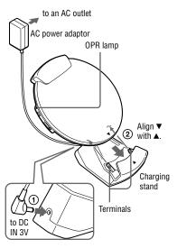
When the battery is completely charged, the OPR lamp goes off and "Charging" disappears.
