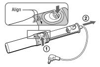
2 Insert an LR6 (size AA) alkaline battery (not supplied) by matching the ⊕ to the diagram inside the battery case. Insert the battery case and lock the case by turning LOCK in the direction of the arrow
