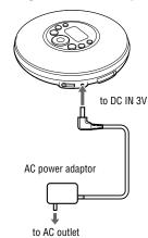
Connect the AC power adaptor to the DC IN 3V jack of your CD player and an AC outlet.
