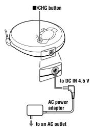
The VIDEO CD player charges the batteries. The "CHG" indicator turns on in the display, and the indicator sections of light up in succession. When the batteries are completely charged, the "CHG" and lindicators turn off. If you press //CHG after the charge has already been completed, the indicator flashes and "Full" appears in the display.
