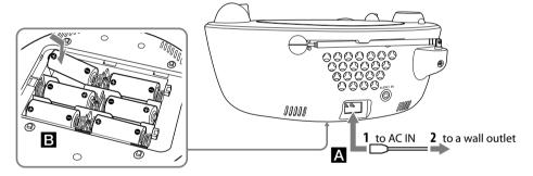
Connect the AC power cord A or insert six R14 (size C) batteries (not supplied) into the battery compartment B.
