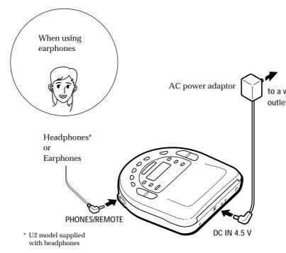
For the models supplied with the AC plug adaptor If the AC power adaptor does not fit the wall outlet, use the AC plug adaptor
