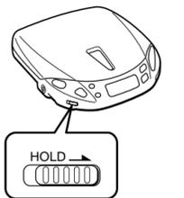
Slide HOLD in the direction of the arrow. When you press any button, "Hold" appears in the display and you cannot operate the player.
