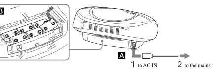
Connect the mains lead A or insert six R20 (size D) batteries (not supplied) into the battery compartment B.
