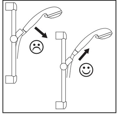
To move the slider up and down the bar, loosen the slider knob. Move the slider to the desired position. Tighten the knob.
