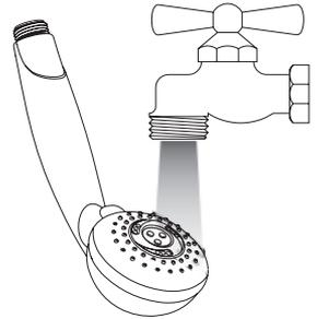
Reinstall the handshower. Turn on the water and allow the handshower to flush for at least one minute.
