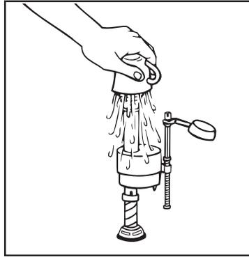
While holding a container over the uncapped VALVE to prevent splashing, turn water supply on and off a few times. Leave water supply off.
