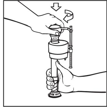
Replace TOP by engaging lugs and rotating 1/8 turn clockwise. MAKE CERTAIN TIP IS TURNED TO THE LOCKED POSITION. VALVE MAY NOT TURN ON IF TOP IS NOT FULLY TURNED TO THE LOCKED POSITION.
