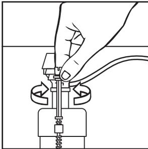
Turn on water supply. Submerge the FLOAT CUP under the water for 30 seconds. Adjust the water to desired level by turning WATER LEVEL ADJUSTMENT ROD and moving FLOAT CUP up or down.
