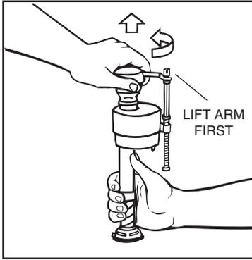
**IMPORTANT: Always clear sand and rust from system.** Make sure water supply is off. Remove valve TOP by lifting arm and rotating top and arm 1/8 turn counterclockwise, pressing down slightly on cap.
