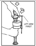
¥ Replace TOP by engaging lugs and rotating 1/8 turn clockwise. MAKE CERTAIN TIP IS TURNED TO THE LOCKED POSITION. VALVE MAY NOT TURN ON IF TOP IS NOT FULLY TURNED TO THE LOCKED POSITION.
