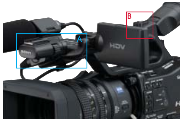
A:Removable Front Shoe B:Screw Hole
