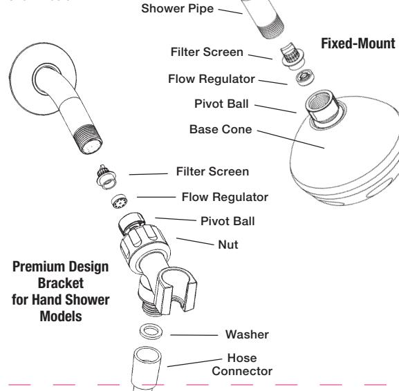
Waterpik® brand showerheads are equipped with an OptiFLOW® regulator that limits maximum water flow to 2.5 gallons per minute at 80 psi as mandated by U.S. federal law.
