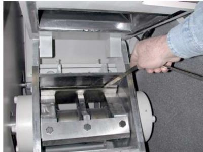
Figure: Checking the knife gap
