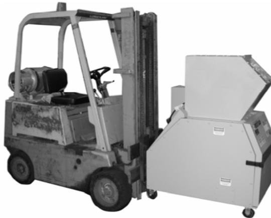
***CAUTION! Do not attempt to lift the granulator with a shaft or protruding member—ESPECIALLY THE HOPPER!***
