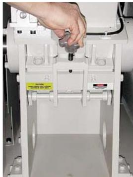
4. Pivot back the feed hopper to gain free access to the cutting chamber.
