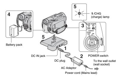
You can charge the "InfoLITHIUM" battery pack (H series) (p. 106) after attaching it to your camcorder.
