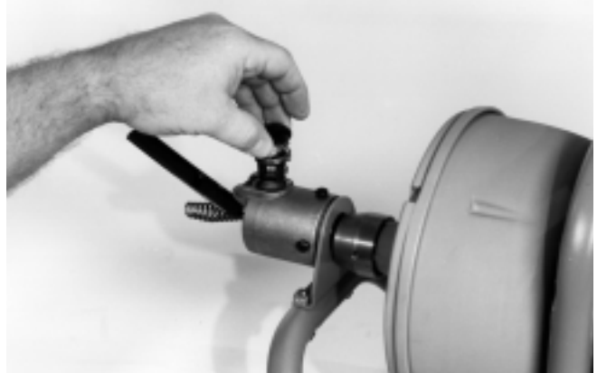
Figure 7 – Autofeed Shown Attached directly to Mounting Bracket
