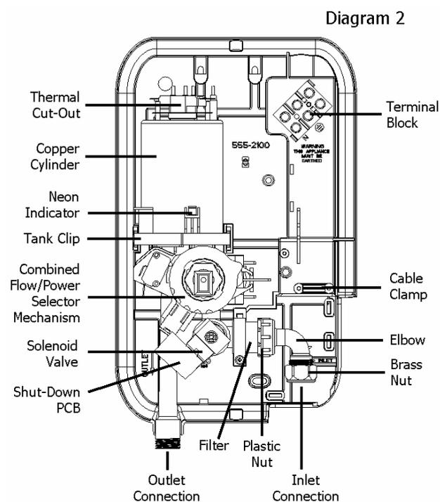
5. If the water supply falls below a set limit, the pressure switch will operate and switch off the power to the elements. This is indicated by the neon light going out (see "Effect of Other Water Devices on Incoming Water Supply").
