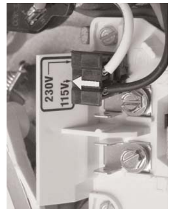
Figure 5B -Voltage Change Plug Set for 115 Volts
