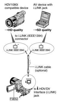
\* i.LINK jack which is compatible with HDV1080i specification is required.
