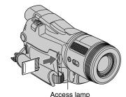
If you force the "Memory Stick Duo" into the slot in the wrong direction, the "Memory Stick Duo," the "Memory Stick Duo" slot, or image data may be damaged.
