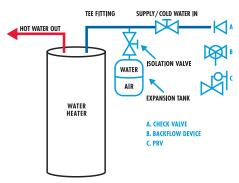
The closed system illustrated requires the thermal expansion tank because of the preceding #2 and #3 facts.
