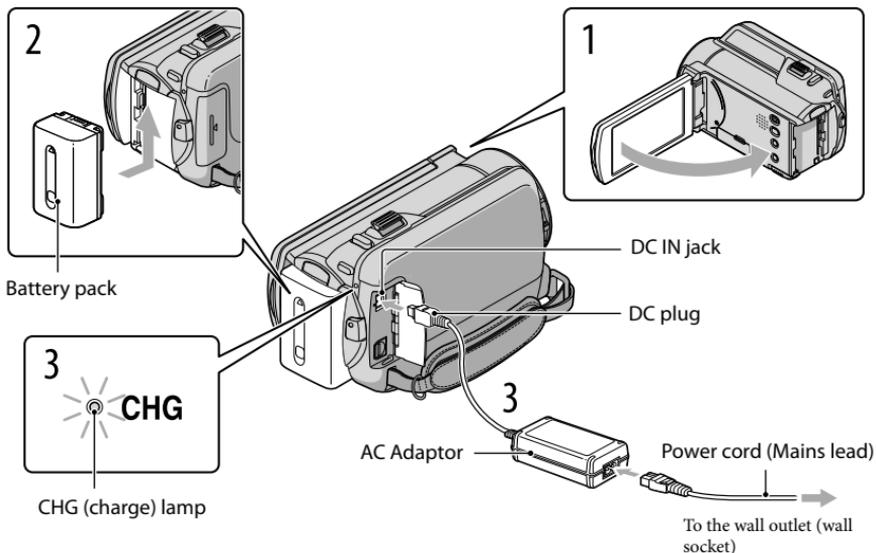
You can charge the “InfoLITHIUM” battery pack (V series) after attaching it to your camcorder.
