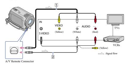
1 Set the input selector of the TV to the input your camcorder will be connected to.
