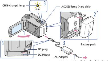
Power cord (Mains lead) To the wall outlet (wall socket)
