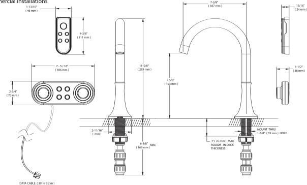
NOTE: THE INSTALLATION SHOWN IS FOR TILE DECKS, THIS VALVE WILL ALSO FIT STEEL, CAST IRON OR PLASTIC DECKS
