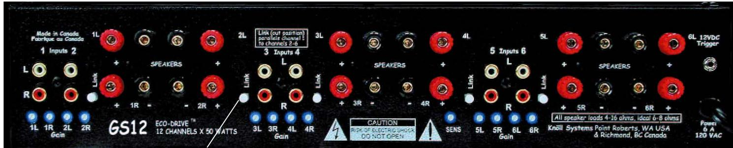
The Link button is normally set to the in position to give all six stereo inputs individual sources. When a channel Link button is set to the out position, that channel is (Left/Right) linked or cascaded to input #1 (without the use of Y cords). Any or all combinations of linked inputs 2 to inputs 6 are possible. When all inputs are linked to input one, the input impedance is about 8500 ohms.
