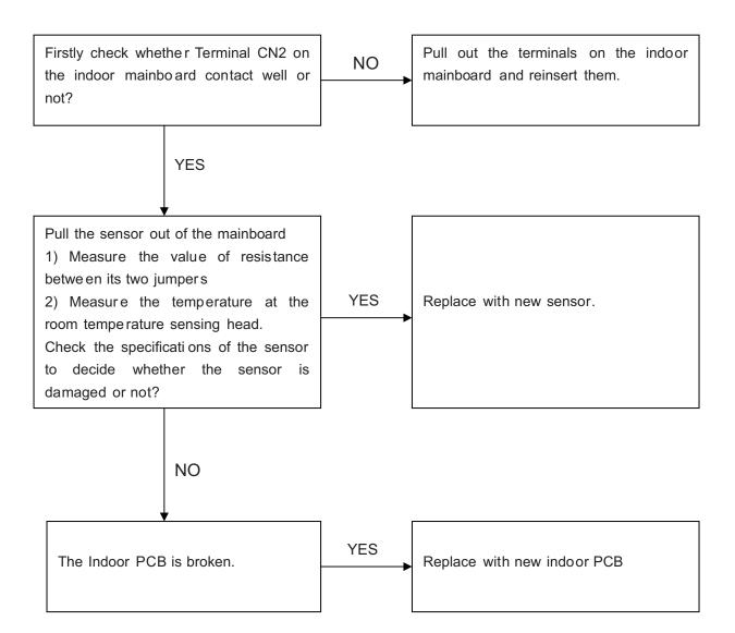
When the unit is ON,the key is failure(ofen ON or OFF),the E2 fault code will be displayed in the temperature indicator and the unit will be stoped .
