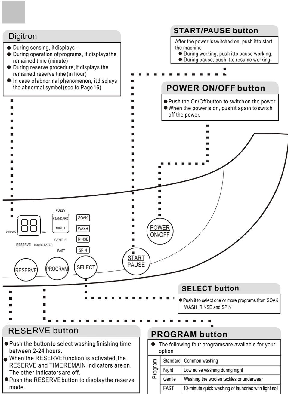
Remarks: Push the On/Off button to switch on the power. If the washing machine is idle for 5 minutes, it will automatically switch off the power.
