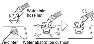
Water inlet valve jointer Water absorption cushion.
