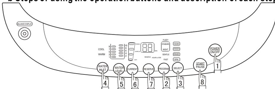
**1 Push the POWER ON/OFF button to switch on the power.**
