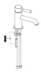
Remove the locking nut and rubber washer from the mounting post.
