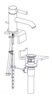
Attach the supply lines to the water supply and check for any leaks.
