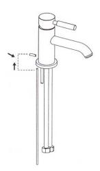
2. Unscrew the handle from the vertical pop-up control rod and then slide the rod through the slot on the back of the mixer body. Then screw the handle back into place.
