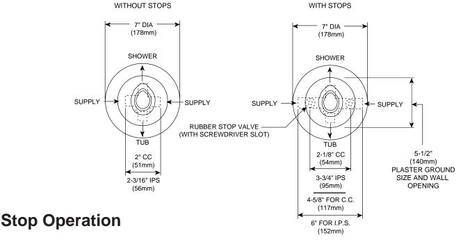
CC - This type is integral with casting, actuated by screwdriver, and require a 90° turn to open or close. When the screwdriver slot is vertical, the rubber stop is closed, and when the slot is horizontal, the rubber stop is open.
