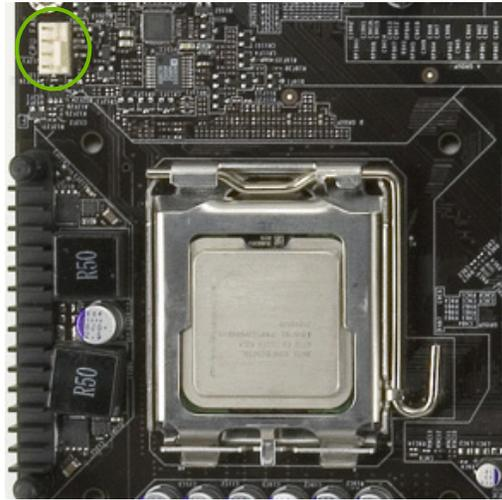
Note that the CPU fan cable can be either a 3-pin or a 4-pin connector. Connect a 3-pin connector to pins 1, 2, and 3 on the motherboard connector.
