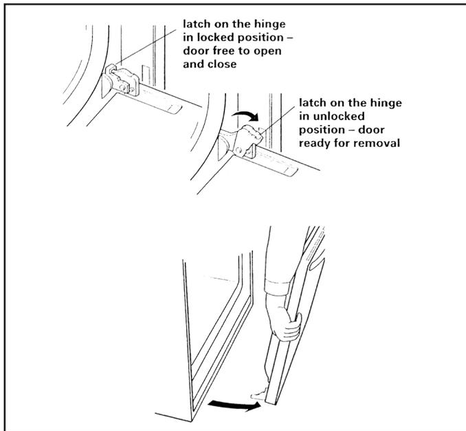
Completely open oven door. In both back corners of the door you will see door latches in the locked position. Rotate both latches forward to the unlocked position.
