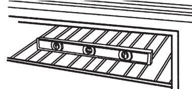
If the range is not level, adjust leveling legs up or down with pliers or your fingers until range is level.
