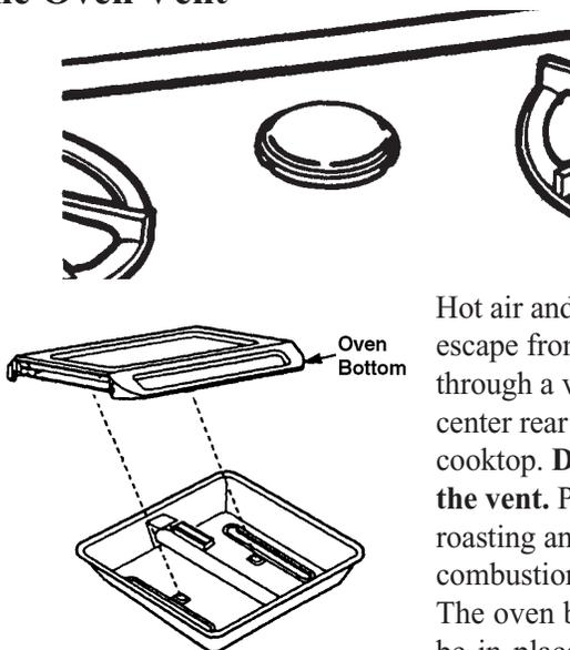
Hot air and moisture escape from the oven through a vent in the center rear of the cooktop. **Do not block the vent.** Poor baking/roasting and bad combustion can result. The oven bottom must be in place for burner to bake properly on model 1956.
