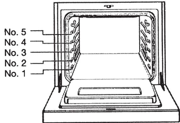
Your oven has five rack positions. Rack position 1 is the lowest position, or closest to the bottom of the oven. Rack position 5 is the highest position, or farthest from the bottom of the oven.
