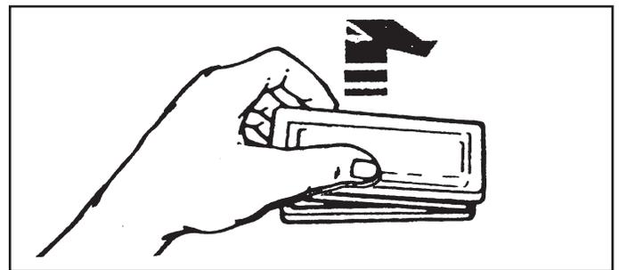
3. Remove bulb from socket. Do not touch bulb with fingers.
