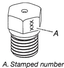
Refer to the following chart for the correct Natural gas orifice spud placement.
