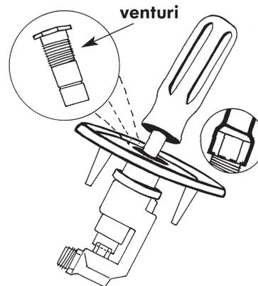
4. Reinstall the brass venturi. Store nat. gas orifices and nut driver so they are available for future conversions. When replacing the black caps, make sure that the tabs in the cap fit into the grooves of the burner base.
