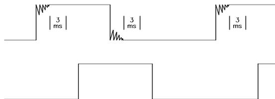
FIGURE 3. SPDT Signal Conditioning by SDM-SW8A
