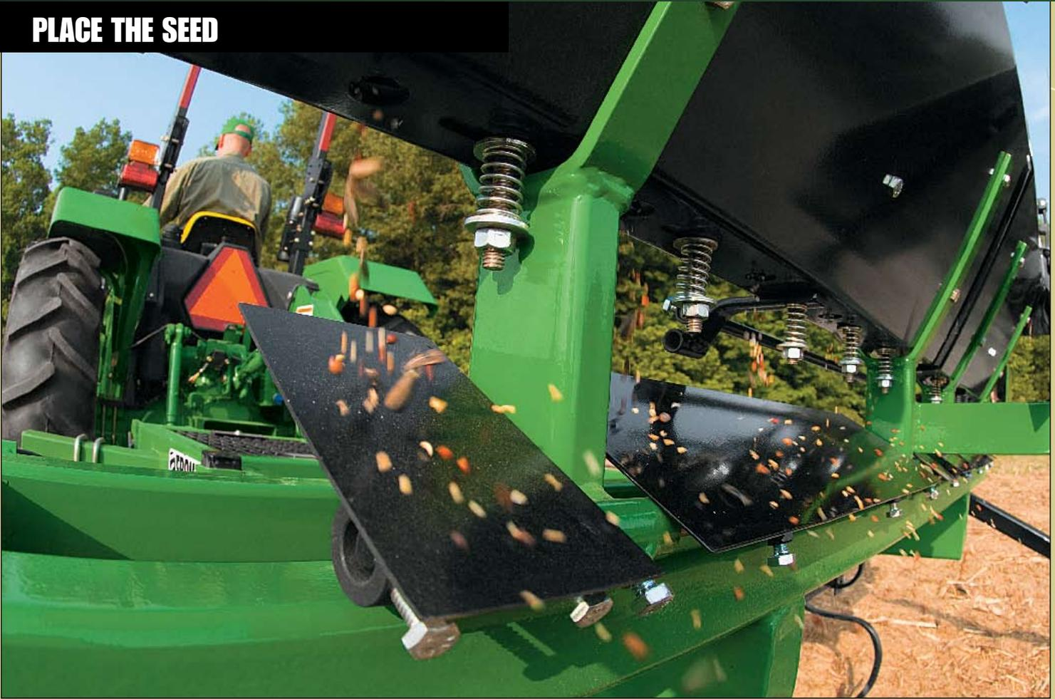
The seed brush (A) allows you to drop almost any kind of seed and will deliver seed, including grass seed and hard-to-plant seed blends, under varied conditions (Seed brush shown without protective shield. Always operate machine with seed brush shield in place). Adjustable scatter plates (B) allow you to set the angle of dispersion for accurate seed placement, reducing seed cost by placing seed only where you want it.
