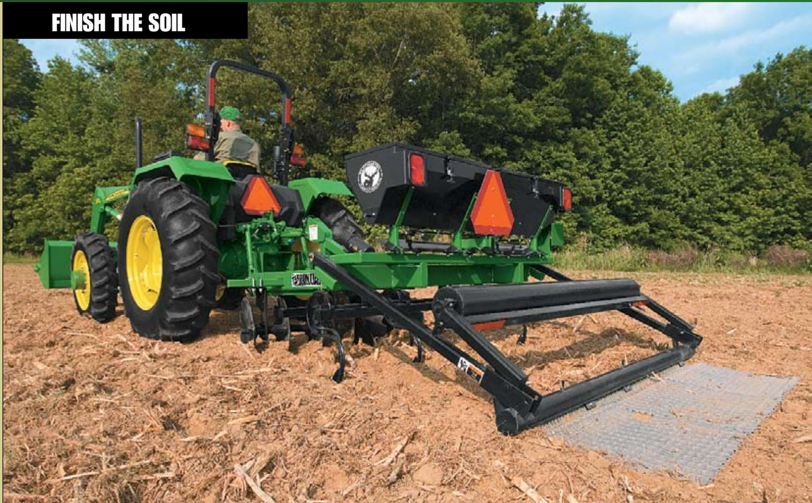
Once the seed hits the ground, the flexible metal grating drag levels the soil and covers the seed for uniform soil contact. You can choose between three covering options. Drag only, drag with roller on top and roller only. The FP1206 and FP1208 feature a handle to easily flip the roller over.
