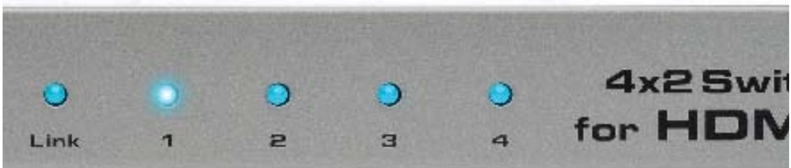
In the illustration above, the LED for Input 1 is blinking and the LED for Input 2 is inactive. This indicates that the Switcher is set to IR channel 1.
