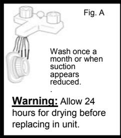
**CAUTION:** The suction hole must be open, free of any obstructions at all times. Otherwise, the motor will overheat and could become damaged.
