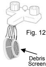
8. Replace the Debris Screen on the HEPA Dust Cup Filter and reinstall filter assembly in the vacuum. (not shown)
