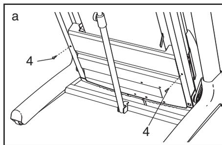
Lower the treadmill (see HOW TO LOWER THE TREADMILL FOR USE on page 25). Remove the four indicated 3/4" Screws (4), and remove the Hood (44).
