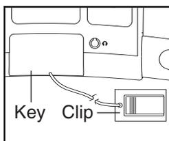
After a moment, the screen will light. **IMPORTANT:** In an emergency situation, the key can be pulled from the console, causing the walking belt to slow to a stop. Test the clip by carefully taking a few steps backward; if the key is not pulled from the console, adjust the position of the clip.
