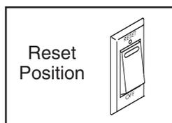
**IMPORTANT:** The console features a display demo mode, designed to be used if the treadmill is displayed in a store. If the screen lights as soon as you plug in the power cord and switch the reset/off circuit breaker to the reset position, the demo mode is turned on. To turn off the demo mode, hold down the Stop button for a few seconds. If the screen remains lit, see THE INFORMATION MODE on page 23 to turn off the demo mode.
