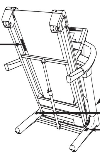
The warning decals shown here have been applied in the locations shown. **If a decal is missing or illegible, see the front cover of this manual and request a free replacement decal. Apply the decal in the location shown.** Note: The decals may not be shown at actual size.
