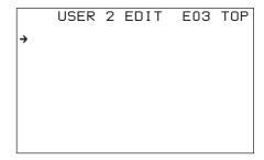
Move the pointer to the item to be added (this operation is unnecessary if no item exists on the page, as shown in the figure for step 3) then push on the MENU SEL/ENTER dial.
