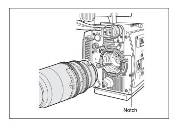
When using an ARRILDS lens or a Cooke /i lens, align the contacts of the lens with a hot shoe of the camera. The camera has two hot shoes that operate completely the same.
