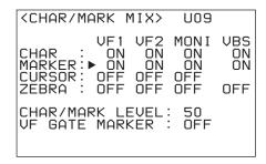
The MARKER indications are activated for all the outputs at the factory.
