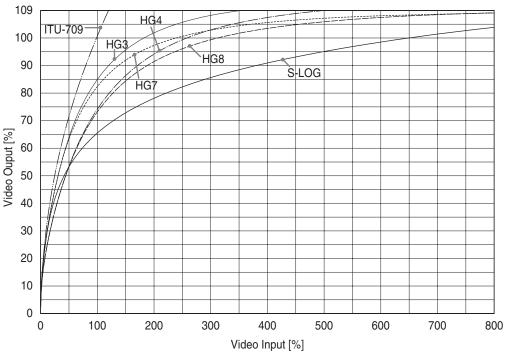
Hyper Gamma curves HG1: HG3250G36 HG2: HG4600G30 HG5: HG8000G36 HG6: HG8000G30
