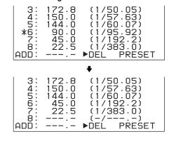
As the numbers for which no value is registered are skipped during a selection operation, deleting step shutter values with lower frequency of use will improve the operation speed.
