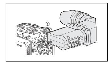
When the supplied center handle is attached to the top of the camera head, you can attach the viewfinder to the viewfinder shoe of the center handle. In this case, first remove the viewfinder shoe from the camera head.
