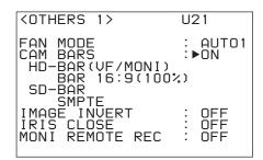
When CAM BARS is set to ON, the color-bar generator is turned ON, and the color-bar signal is output.
