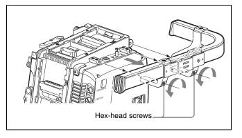
To attach the handle in the original position, reverse the procedure for detaching.
