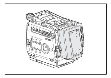
**7** Rotate the accessory clamp lever downward (toward the opposite direction of the lens when attaching to the top).
