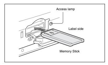
If it does not fit into the slot properly or if there is some resistance when you insert it, the "Memory Stick" may be turned around or upside-down. Do not force the "Memory Stick" into the slot. Confirm the direction of the notch and arrow on the "Memory Stick" before inserting the "Memory Stick," and then try inserting it again.
