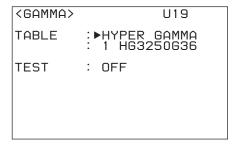
2 Observing the output video level for a gray card of 18% reflection rate on a waveform monitor, adjust the iris so that the level becomes equal to that shown in the "Video output with 18% gray card" column of the "Available Hyper Gamma choices" table. (The iris setting in this condition is the standard iris setting for the selected hyper gamma.)
