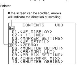
Turn the MENU SEL/ENTER dial to align the pointer with the desired page indication then push on the MENU SEL/ENTER dial.
