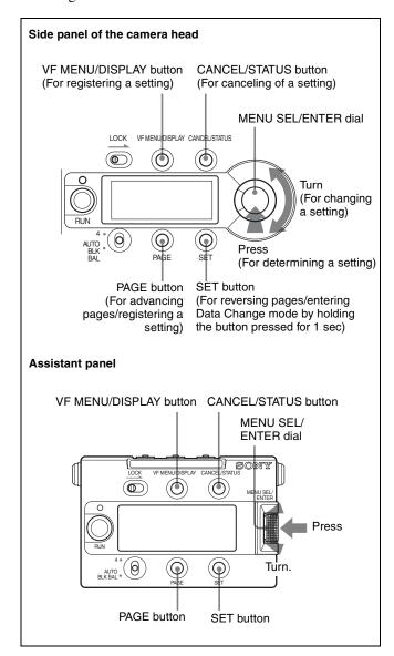
Operations of the subdisplay are possible with the buttons and dial both sides of the camera and assistant panel.
