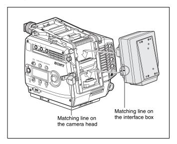
**5** Rotate the accessory mount lever downward (pull it in the opposite direction of the lens when attaching to the top).
