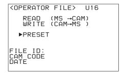
Position the pointer to PRESET and push on the MENU SEL/ENTER dial. The operation items return to the statuses stored in the operator file.
