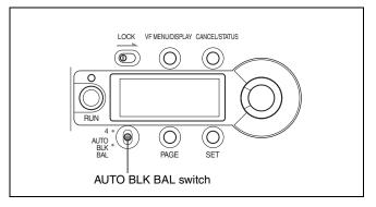
During adjustment, "ABB: EXECUTING" is displayed on the viewfinder screen. When the adjustment process is completed successfully, the message "ABB: OK" is displayed.
