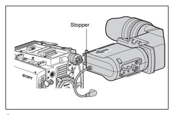
2 Set the viewfinder to the most convenient position, tighten the viewfinder positioning ring (1) in the figure below), and connect the viewfinder cable to the VF1 connector of the camera (2) in the figure below).
