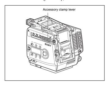
Release the lock by sliding the lock-release knob in the direction of the arrow (① in the figure below) then pull up the accessory mount lever (pull it toward the lens when mounting on the top) (② in the figure below).
