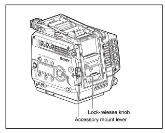
4 Aligning the matching line on the interface box with that on the camera head, fit the interface box into the camera head then push down on the box (slide it in the opposite direction of the lens when attaching to the top) so that the connectors engage.
