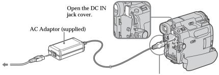
Connect the plug with its **A** mark facing the battery.
