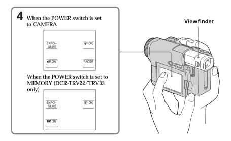
To make the buttons on the LCD screen disappear  $Press \Rightarrow OK$ .
