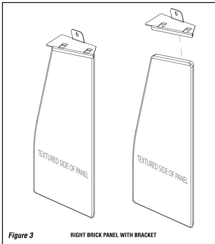
**Step 4.** Repeat step 3 using the left brick panel bracket and left brick panel.
