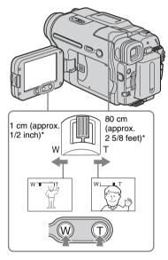
\* The minimum distance required between your camcorder and the subject to get a sharp focus in that position of the lever.
