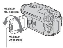
Press OPEN and open the LCD panel.
