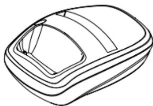
Plug the charger into a wall outlet and plug the connector (on the charger lead) into the back of the Compact Desktop Charging Stand. Place your phone and/or a spare battery in the stand to begin charging.
