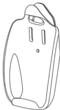
When you need to remove the phone from the holster, gently press the release tab on top of the Belt Holster away from the phone and tilt the phone forward.
