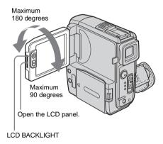
Open the LCD panel 90 degrees to the camcorder, then rotate it to the desired position.
