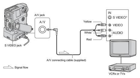
\* By using an S video cable (optional), higher quality DV format pictures can be produced.
