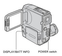
You can check the battery's current charge level and its current remaining recording time both during charging or when the power is turned off.
