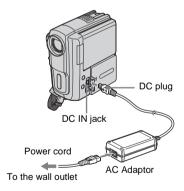
You can charge the battery pack on a trip, even if you have not brought the Handycam Station along. With the ▲ mark on the DC plug facing up, connect the AC Adaptor to the DC IN jack on your camcorder as shown in the illustration.
