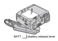
Attach the battery pack with its terminal side facing your camcorder as shown in the following illustration and press down the battery pack until it clicks.
