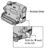
If you force the "Memory Stick Duo" into the slot in the wrong direction, the "Memory Stick Duo," the "Memory Stick Duo" slot, or image data may be damaged.
