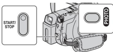
① Set the POWER switch to **🎬** (Movie), and press START/STOP to start movie recording.
