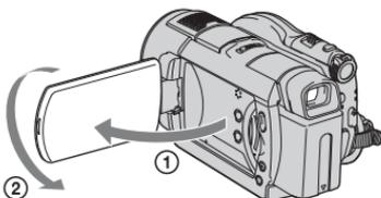
Open the LCD panel 90 degrees to the camcorder (①), then rotate it 180 degrees to the lens side (②).
