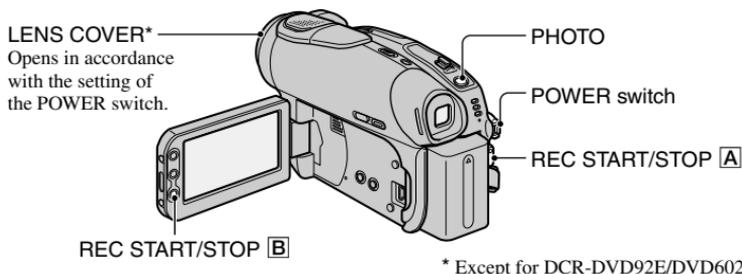
**1** Slide the POWER switch down repeatedly to light up the respective lamp.
