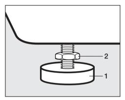
Using the spanner supplied turn counter nut 2 in a clockwise direction. Then turn counter nut 2 together with foot 1 to unscrew.
